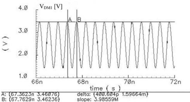
Fig. 7. Drain voltage waveform of transistor  $M1$   $V_{DM1}$ .
