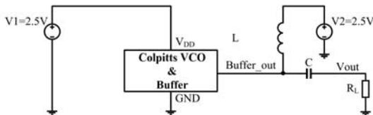
Fig. 6. Simulated Colpitts VCO and buffer block circuit.
