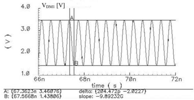
Fig. 8. The peak-to-peak voltage of  $V_{DM1}$ .
