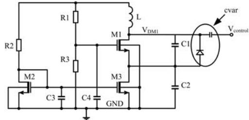
Fig. 13. Schematic of Colpitts VCO core with varicap.
