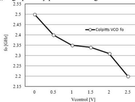
Fig. 14. Frequency of oscillation  $f_o$  of Colpitts VCO as function of control voltage  $V_{control}$ .
