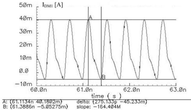
Fig. 11. The waveform of drain current of transistor M1 ( $I_{DM1}$ ).
