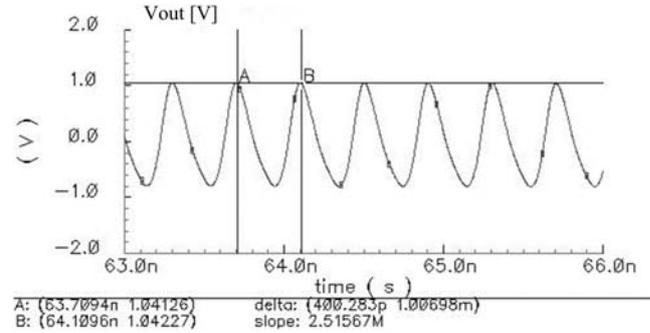
Fig. 9. The simulated waveform of output voltage  $V_{out}$ .
