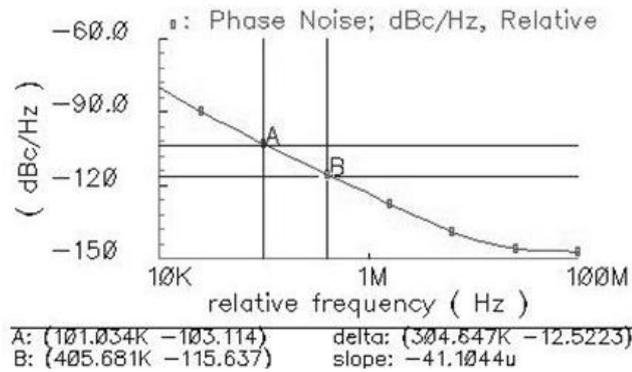
Fig. 12. Phase noise characteristic of designed Colpitts VCO.
