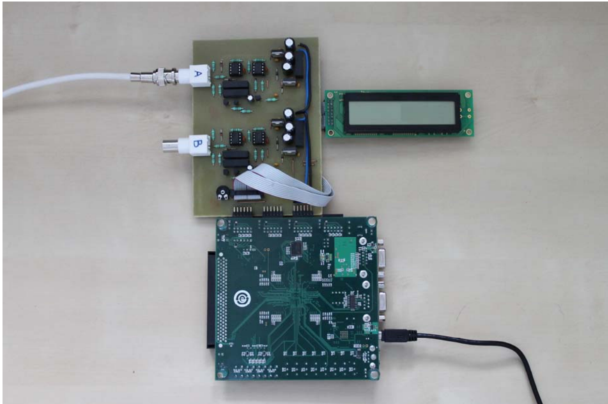
Fig. 8. Developed board with input attenuators, input stages, power supply, ADC and LCD display
