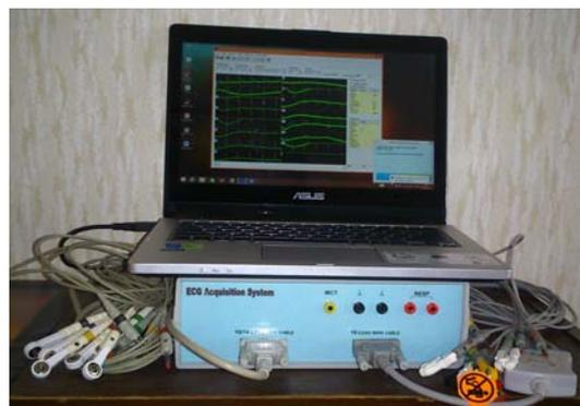
Fig.3. ECG acquisition module connected to PC
