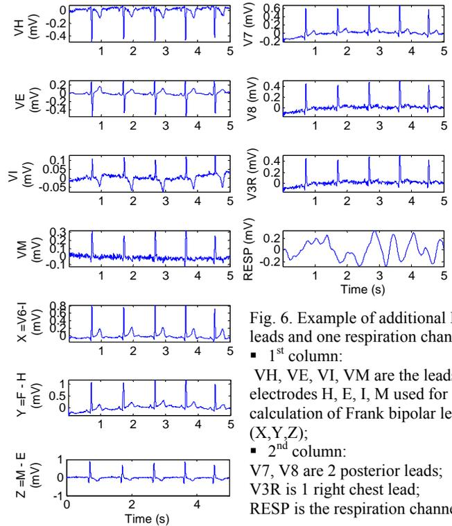
Fig. 6. Example of additional ECG leads and one respiration channel:
