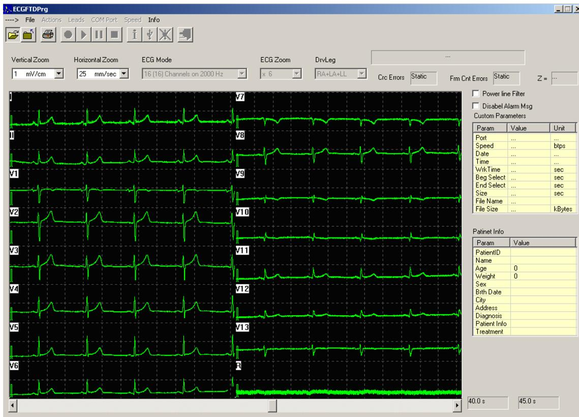
Fig. 2. Main window of the PC application for management of the real-time signal acquisition, recording and visualization of multi-lead ECG (I, II, V1-V6 (standard), V7-V13 (additional)) and one respiration channel (R).
