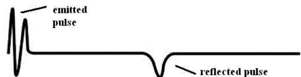
Fig. 2. Short-circuited line reflection
