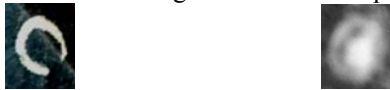
Fig. 3. Actual photograph of the laser spot of the beams emitted from the external part (blocked internal) – left and of the simultaneous operation of the both parts -right
