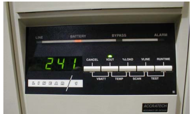
Fig. 4. UPS front panel
