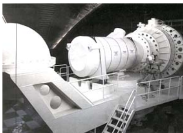
Fig. 2. Optical telescope of the laser-optical component.
