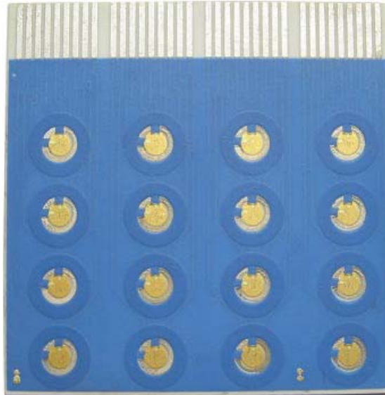
Fig. 5: The real sample of electrochemical sensor array.
