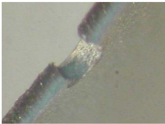
Fig.11.: Detail of defect in the hole (bad adhesion of deposited silver thin film layer to the substrate)
