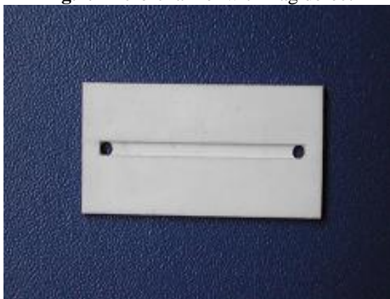
Fig.4.: Detail of micro-channel with holes
