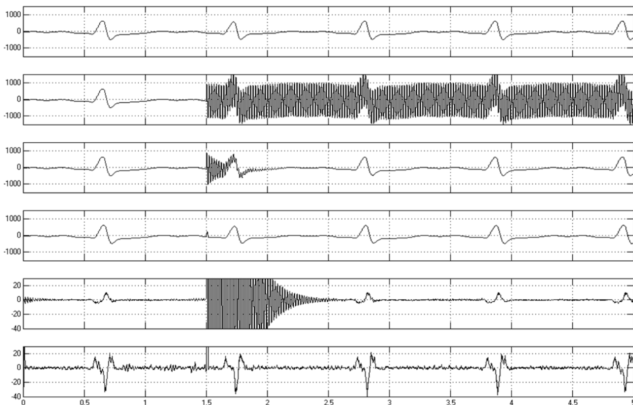
Fig.7 Simulation results of cascaded comb filter compared with one PL period (20 ms) averager
