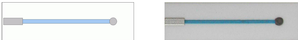
Fig. 2 Working electrode substrate design (left) and its real sample (right).
