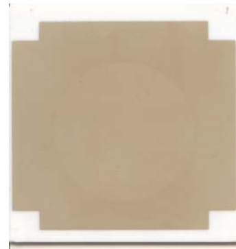
Figure4. Photomask for second screen printing Figure5. Substrate after second screen printing-photography
