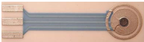
Fig. 2: The TFT amperometric sensor with graphite working electrode without AgCl layer deposited over the reference electrode.
