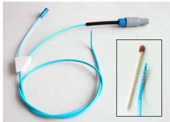
Figure 3. Catheter for in-vivo characterization of blood in the right atrium.
