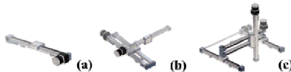
Fig. 1 Models of the DriveSets -family instances (a), (b), (c)
