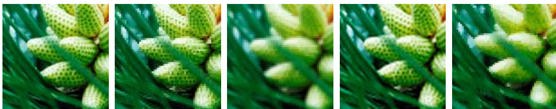
Fig. 6 From left to right: (a) – ROI on test image PineCone, (b) – NN, (c) – SI, (d) – BSI a = -1 , (e) – DDT
