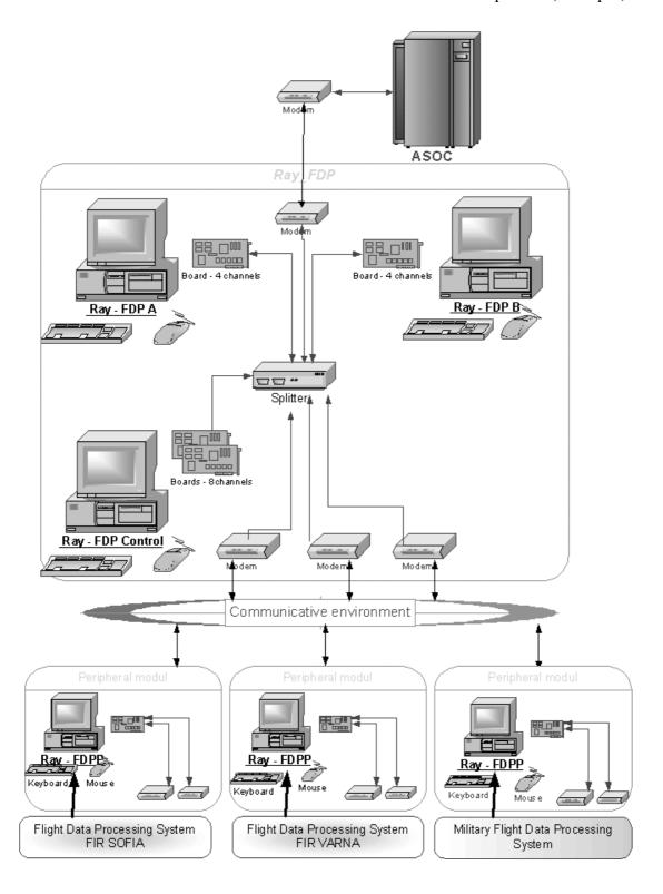
Fig. 2. Structural diagram of System for Integration of Civil and Military Flight Plans for Aims of ASOC.
