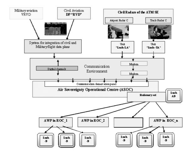
Fig. 1. Structural shame of the systems developed by the scientists of SRI-BAS used for the creation of ASOC
