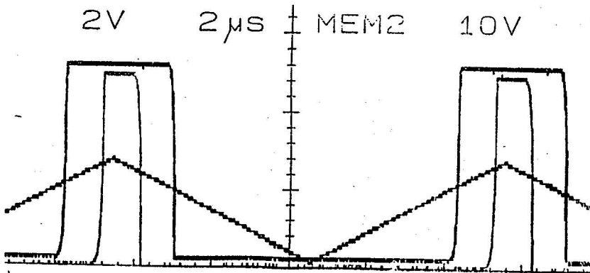
FIG.7. EXPERIMENTAL WAVEFORMS OF THE ANALOG INPUT AND TWO ADC COMPARATOR OUTPUTS
